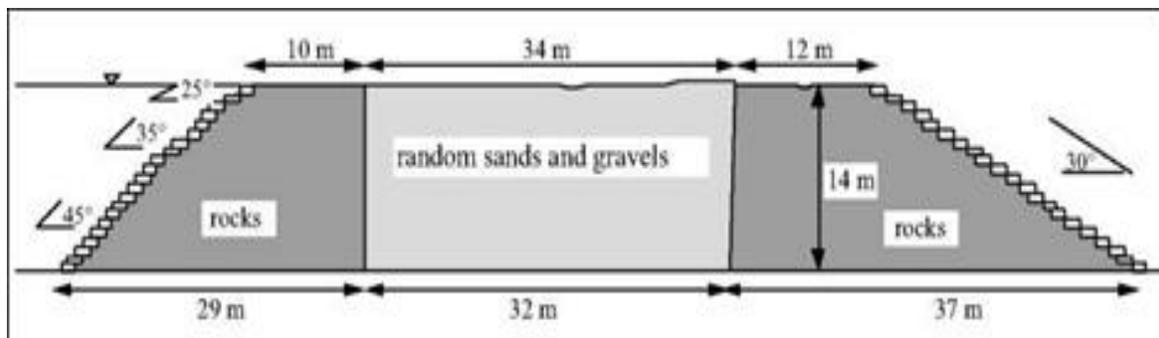
Fig.1. Note. Cross section of the structure of the Sadd el Kafara dam. From Sadd-el-Kafara: the world's oldest large dam. International Waterpower & Dam Construction by G. Garbrecht, 1985, *International Water Power & Dam Construction*, 37, p. 74.
